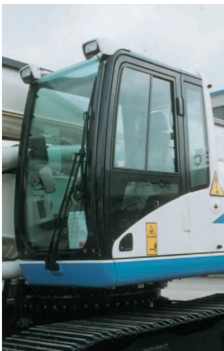
The new R-620 is installed on new "Caterpillar" turret with easy access to any hydraulic and mechanical parts. New designed cabin allows better visibility and easier way of use.
